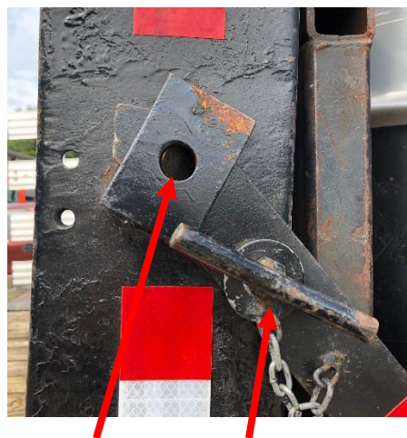
Latch Pin & T-Bolt Secure the Horizontal Safety Bar
