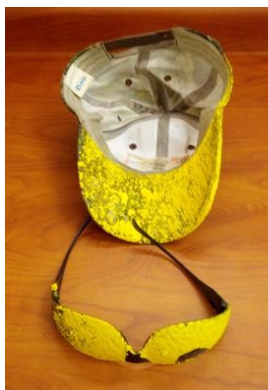
7/14/2012 Spray Thermoplastic material sprayed in the face of the person working on the STP gun tip that was under pressure.
