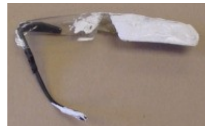
10/30/2003 Epoxy flush discharged in the air hitting the employee in the face. The material melted the safety glasses.
