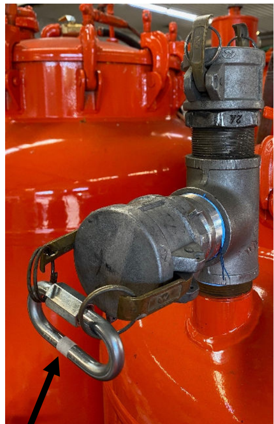
Oval Threaded Link securing the cam-lock cap.
